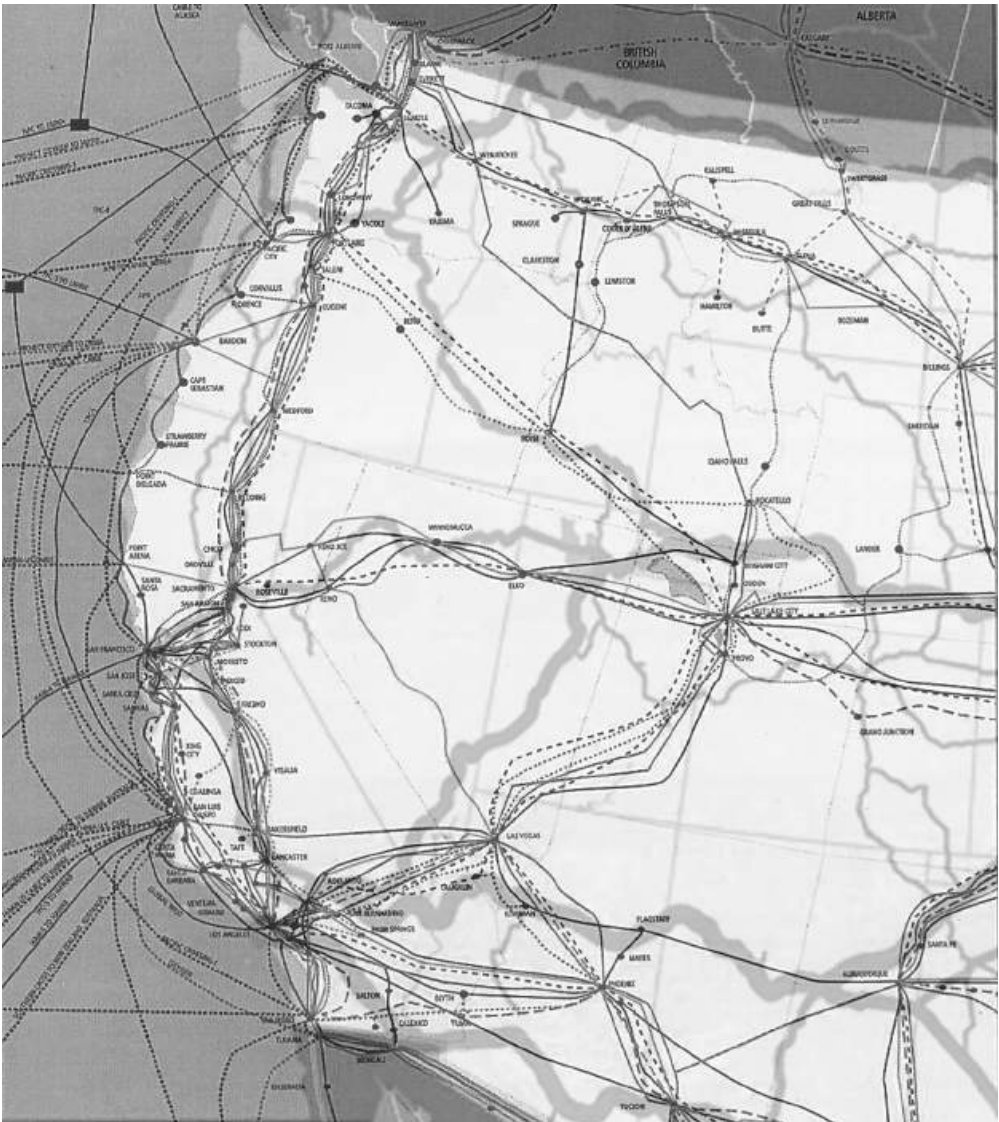
Figure 1.2 Overlay of fiber-optic routes and railroad routes. Sources: KMI Corp., “North American Fiberoptic Long-Haul Routes,” 1999; U.S. Department of Transportation, Federal Railroad Administration, 2010. (KMI was acquired by CRU Group, crugroup.com, in 2006.)
